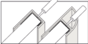
End trims and Quadrant trims Finishing end trims for square cut edge panels.
