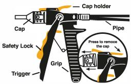
**5.** Point the gun to the surface to be sprayed at a distance of 6-22 inches (15-60cm). The polyurethane foam will swell and complete the reaction in about 60 seconds. Make sure that the cap holder is closed before spraying as shown in the figure below. If you are going to spray for more than 30 seconds, replace the cap with a new one.
