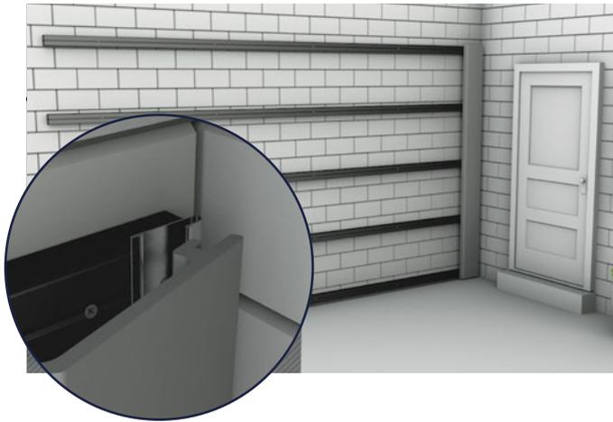
**5** Secure the Boards using a screw at least 30mm in length, ensuring that the Board is fastened securely on each Batten that it touches. Secure these fixings by hand, as it is important not to over-tighten the screws and risk splitting the Board.
