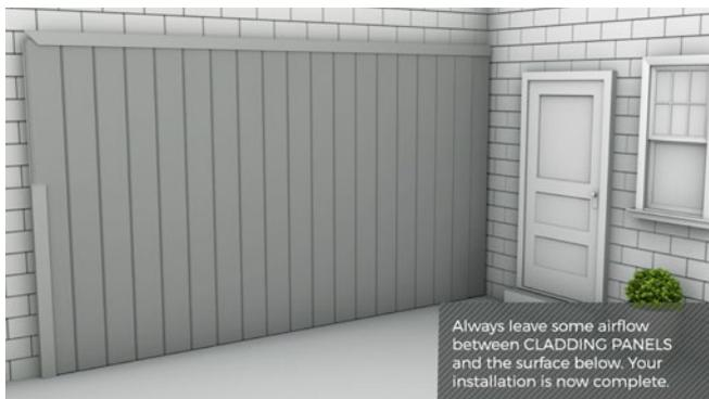
**8** Depending on your installation, you may want to finish off the edges using one of the Trims Cladco can provide to give you a lasting professional look. There are a range of Trims available in all colours to complement your Cladding Boards, which can be secured to your installation by glue, using an exterior grade high elastic glue.
