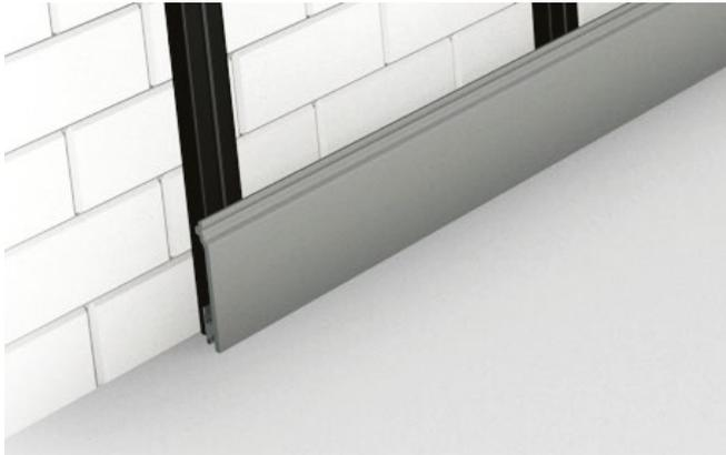
**4** Secure the Boards using a screw at least 20mm in length, ensuring that the Board is fastened securely on each Batten that it touches. Secure these fixings by hand, as is important not to over-tighten the screws and risk splitting the Board. Ensure that the section between the Battens remains empty allowing air to flow beneath the Boards.
