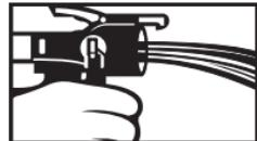
4. Purge the system into a waste container by activating the trigger of the Insta-Flo™ dispenser.
